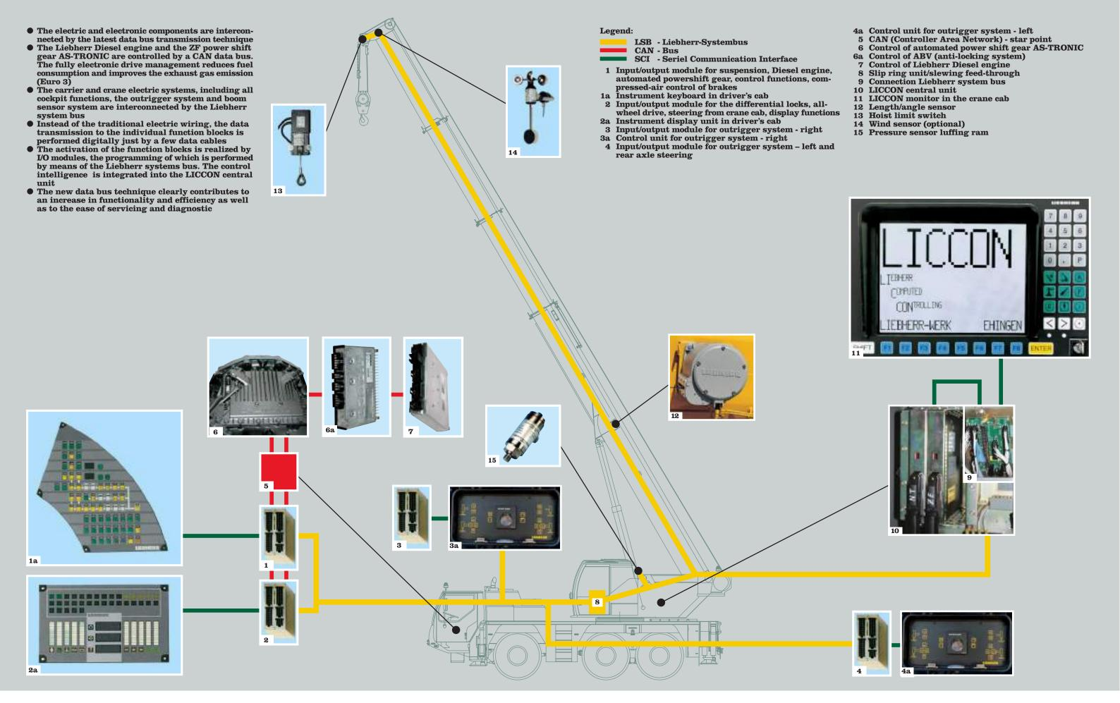
Data bus technique revolutionizes crane electric system.
